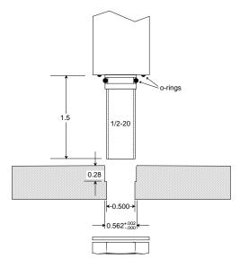
Figure 3. Drawing of bulkhead sensorand customer housing.
