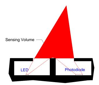
Figure 2. Diagram of Seapoint Turbidity Meter Optics
