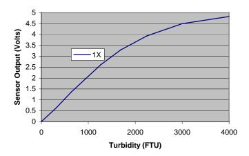
Figure 4. Sensor Response to Formazin Turbidity Standard
